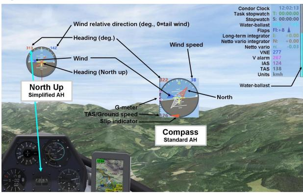
The text window shows (bottom to top): Velocity units, TAS, IAS, Alarm velocity, VNE, Netto Variometer (n), Netto Variometer Integrator (N), Total-energy long-term Integrator Variometer<sup>2</sup> (I), Water-Ballast (WB), Flaps settings (Fl), Stopwatch (S), Task stopwatch (T) and Condor clock
